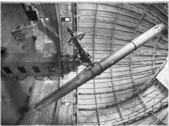
THE LARGEST REFRACTOR, THE 40-INCH TELESCOPE AT YERKES OBSERVATORY. DOME 90 FT. IN DIAMETER. (Photo, Yerkes Observatory.)
